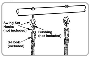
Fasten the Lift & Lock Swing S-hooks (included) onto the hooks (not included) on your swing set.
